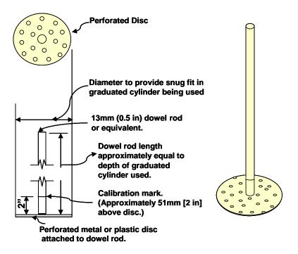
Note: The perforation in the disc should be small enough to permit the passage of any small floating particle.
